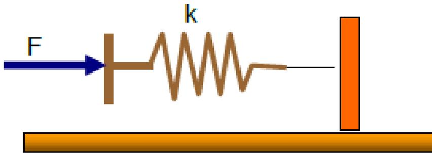
$$F = k x \quad k = \frac{F}{x} \quad k = \frac{20 \text{ [N]}}{0,1 \text{ [m]}} \quad k = 200 \text{ [N // m]}$$
